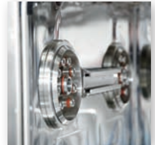
Cart/washing machine coupling system.
